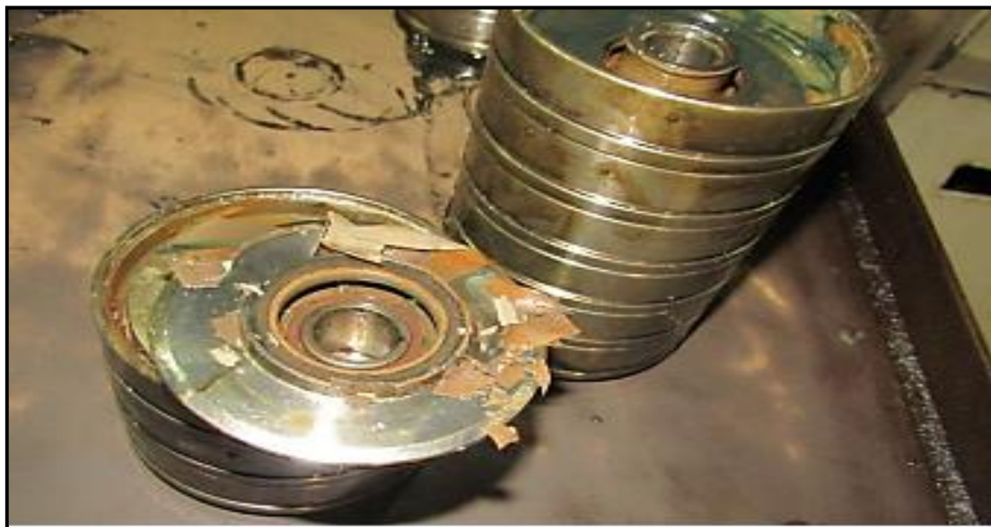
Figure 2 – Salt deposits in the working organs of EOTS
