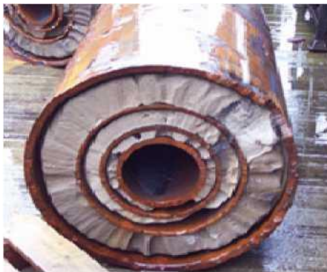
Figure 1 – Gaps between columns and cement stone
